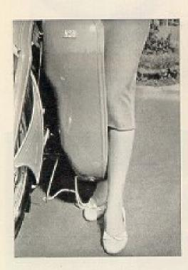
Another point to note; the smart NSU leg shields can be fitted to any Quickly, and this transforms the moped in a moment into a vehicle offering the smartness and the protection of a scooter.
