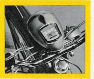
Moped drivers should know how fast they are travelling and how many miles they have already covered. The Quickly-S has, therefore, been provided with a speedometer, which is built into the headlamp.
