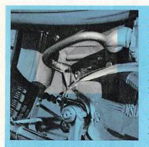
And to add to its smart appearance, the machine has chromium plated rims. Another useful addition is the convenient handle on the right-hand side of the Quickly with which it can easily be lifted and, for example, carried up a flight of steps or over an obstacle. The exhaust pipe is on the right-hand side, a particularly thoughtful piece of design, so that there is no danger of touching it while carrying the machine.
